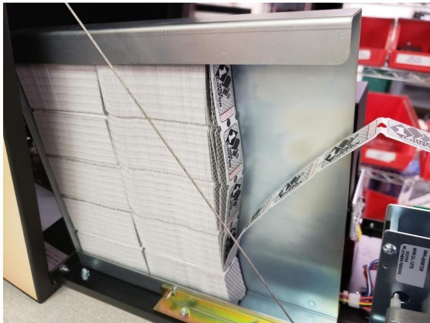
Place fanfold tickets into the hopper as shown.
