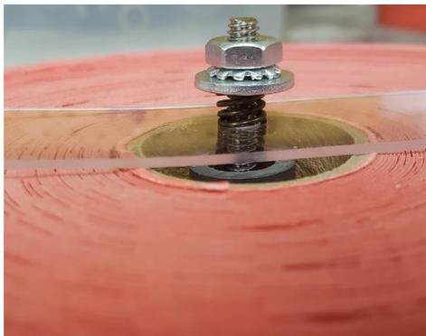
Install the spring, washer and nut on the screw to hold the plastic guard in place.
