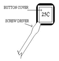
PLACE THE SCREW DRIVER AT THE EDGE OF THE BUTTON COVER AND TWIST THE DRIVER UP. REPEAT THIS FOR THE REMAINING EDGES.
